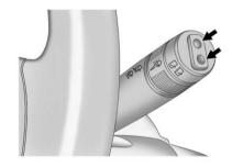
Press the upper or lower portion of the button to control the rear wiper and rear wiper delay.
